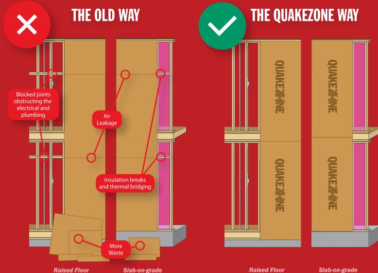
Get the wall sheathing that allows you to build faster while still meeting code. QuakeZone is the right size for the way you frame, allowing you to build faster and increase productivity.
