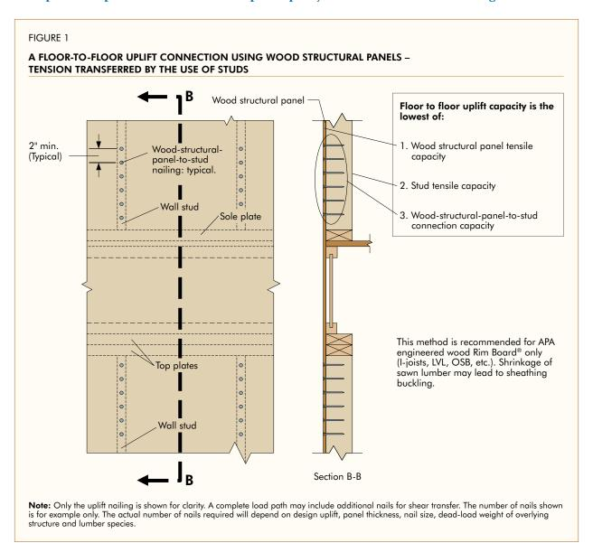
Assume: Sheathing is 7/16-inch oriented strand board (OSB), APA Rated Sheathing (24/16 Span Rating), oriented such that the tensile stress in the panel is perpendicular to its strength axis; the shear wall must resist 500 lbf/ft of wind uplift force; 6-8d common nails per stud are used as shown; wall framing is Stud grade 2x4 Douglas-fir; and stud spacing is 16-inches o.c.
