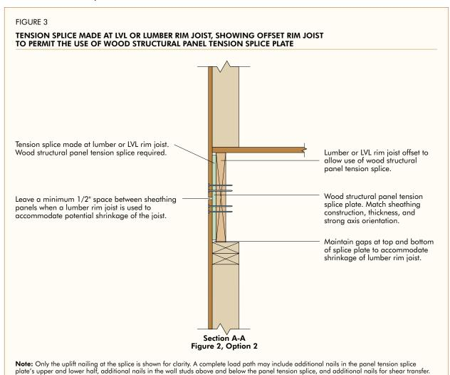
Number of nails shown is for example only. Actual number required will depend on design uplift, panel thickness, nail size, dead-load weight of
