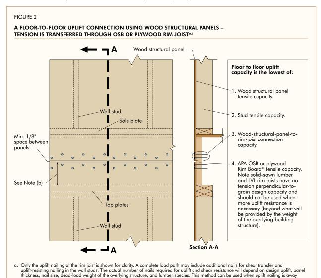
b. Figure above shows panel overlap at middle of rim joist. Minimum sheathing-over-rim-board overlap is 1-1/2". Such an overlap is sufficient to support two rows of 10d (0.131" x 2-1/2") nails, each row at 3" on center, while maintaining a minimum panel edge distance of 3/8".
